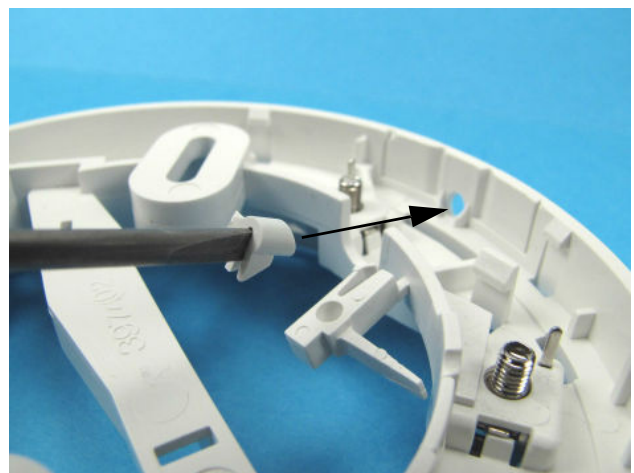
Fig. 4: Inserting the LED aperture plug
