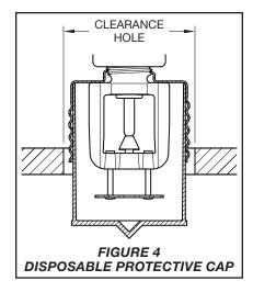
**Step 5.** Replace the Protective Cap by pushing it upwards until it bottoms out against the Support Cup. (Ref. Figure 4.)
